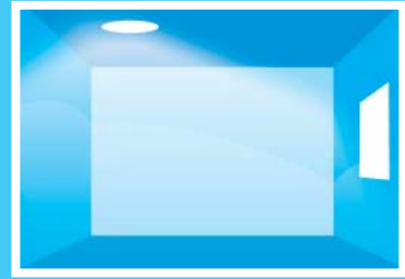
light tunnel placement in a room with a window. The placement of a light tunnel too close to a wall opposite to a window may diminish the overall light in the middle zone.
